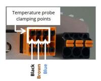
If more than one probe is used, the cores can also be connected externally in parallel.
