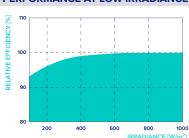
Typical module performance under low irradiance conditions in comparison to STC conditions (25°C, 1000 W/m²).
