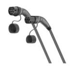
Charging cable for up to 11 kW charging capacity @ 3-phase connection, plug type charging station: type 2, plug type electrical vehicle: type 2, 7.5 m cable length, plug colour black/grey, cable colour black
