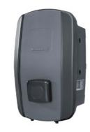
Mode 3 EV-charging box AC SMART ADVANCED, max. charging power of 11kW at 3-phase (400 V) mains connection, maximum charging current 16 A, attached 5/7.5 m cable with type 2 plug, RFID authentification, MID compliant energy meter, integrated webserver with dynamic load management, mobile App, Interfaces: mobile communications (4G/LTE), 2x Ethernet, WLAN, Bluetooth LE, RS 485, 5 DI, 1 DD, powerline communication (AutoCharge)
